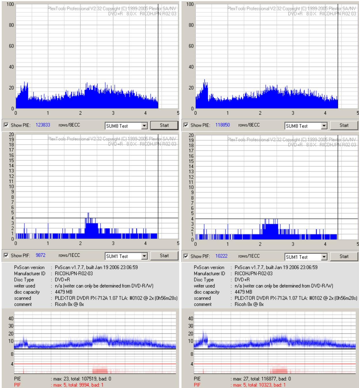
Figure 8: Scan of a physically damaged disc - before and after
