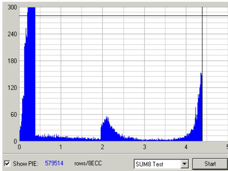
Figure 1: PIE scan with PlexTools Professional v2.17 of a bad recording
